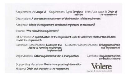
Figure 1 The Volere shell for capturing requirements
